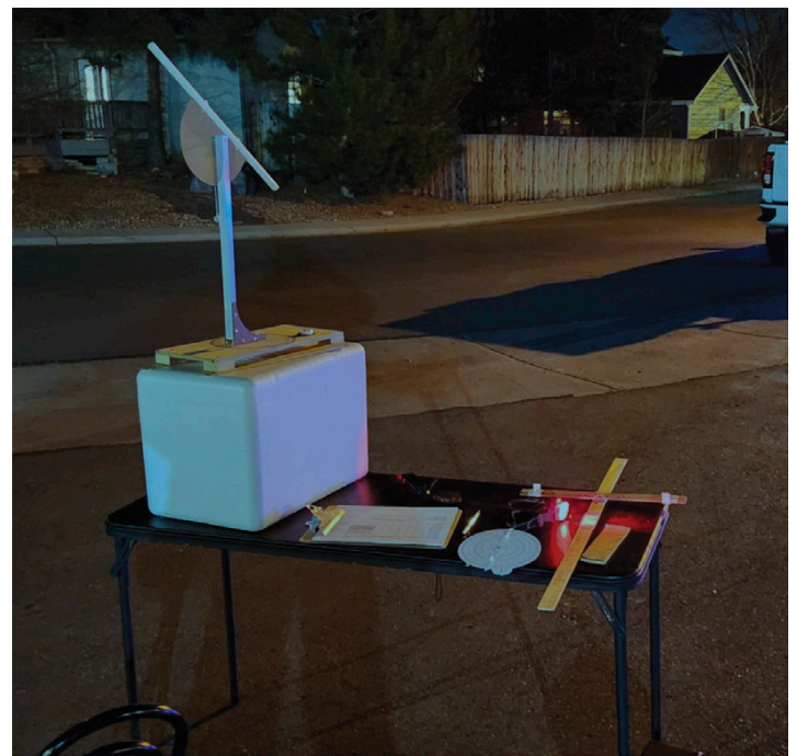
Using Quadrant and Jacob's staff to site Polaris at night
